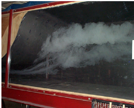
Fig. 1. Flow visualization with smoke.
